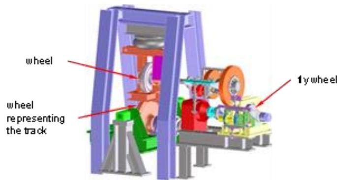
Figure 1: CAD-Model of the Single-wheel Rolling Testbench
